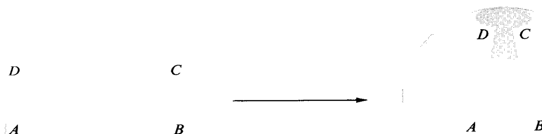
FIGURE 12.3 Deformation of a rectangle into a hemisphere.
